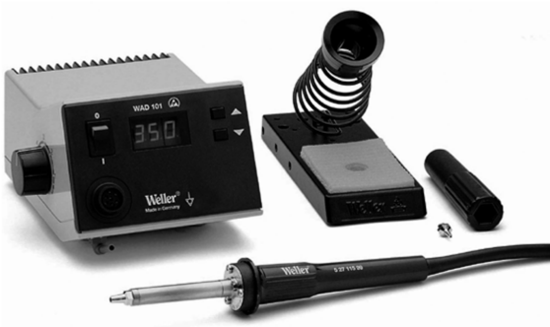
Figure 6-7. Simple Weller WAD101 rework station (reproduced with permission)
